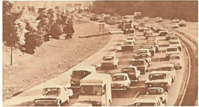
Level of Service E: Unstable flow of traffic, with volumes at or near the capacity of the highway, resulting in stop-and-go operation of vehicles.
