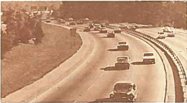
Level of Service B: Stable flow of traffic, with drivers still having reasonable freedom to select lanes and maintain desired speeds.
