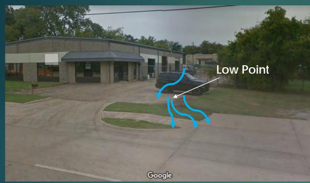
Photo Prior to project; private property had stormwater from parking lot drain over sidewalk into street
