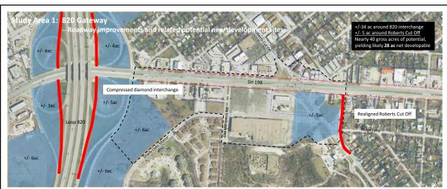
The 820/199 cloverleaf interchange occupies a large land footprint that may be converted into an urban diamond interchange in order to provide for a new development gateway to the 199 corridor.
