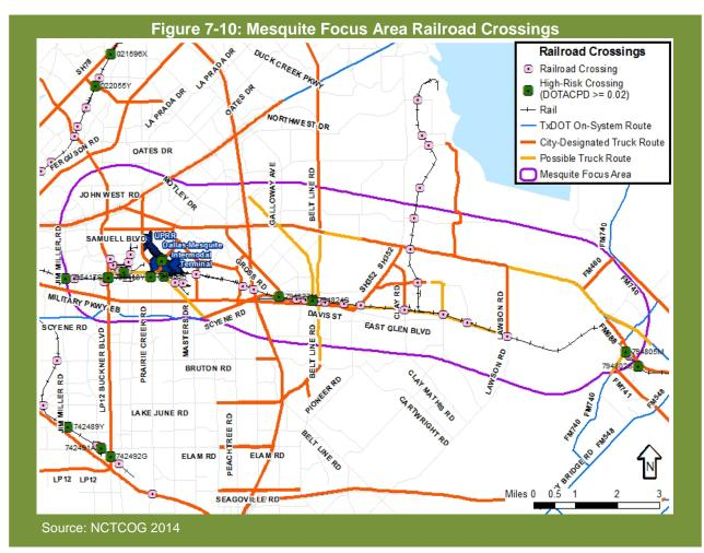
FRA data indicates 20 trains use the UP line daily. The railroads are grade-separated at crossings where rail lines cross major highways and roads such as IH 635 and Loop 12. The at-grade crossings on the UP line along SH 352 are not directly on the truck route but can still impact movements. Two of these crossings are considered high-risk crossings by the DOTACPD. Two crossings along the truck route on SH 180 and the UP, are also considered high risk by the DOTACPD.
