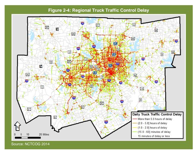
Traffic control delay is an issue throughout the region. With most traffic control delay occurring within the first or last mile, the benefits of optimizing traffic control systems are much more localized.
