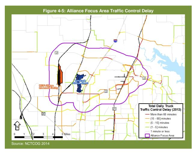
Since traffic control delay occurs mostly near the beginning or end of a trip, the benefits of optimizing traffic control systems are much more localized. The estimated results show highest traffic control delay along Westport Parkway/Keller-Haslet Road and on US 377. Additional roads with traffic control delay include Alliance Boulevard at IH35W, SH114/ IH35W Interchange, and Eagle Parkway at IH35W.
