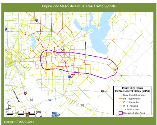
Since traffic control delay occurs mostly near the beginning or end of a trip, the benefits of optimizing traffic control systems are much more localized. The estimated results show highest traffic control delay along SH 352 near US 80 and Belt Line Road near US 80. Additional roads with traffic control delay include Galloway Avenue and Loop 12 near IH 30.
