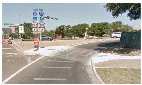
Figure 4: Example of a raised crosswalk on a turn lane joining an interstate frontage road in Austin, TX. (Source: Google Street View https://goo.gl/maps/PnLAq25X2tKVjf8e9)
