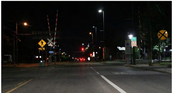
Figure 6: Crosswalk near the DART station. The addition of pavement markings and a right-side warning sign would increase conspicuity for drivers, particularly at night.
