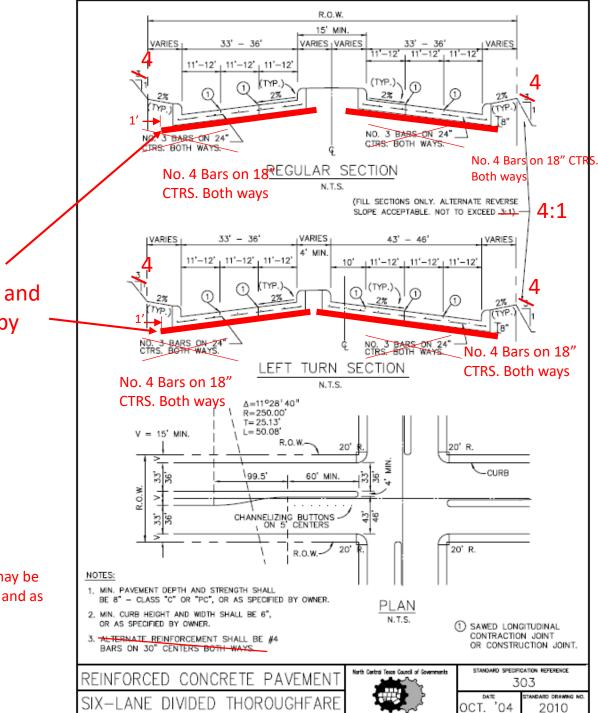
Replace Plan with a more general layout to include crosswalks, ADA ramps, striping, and possibly additional lane width for bicycle lanes per TxDOT 8" minimum stabilized subgrade per section 301 and as approved or specified by owner
