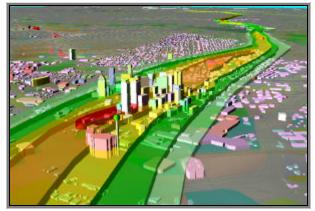
*Figure 2.* Modeling GIS data of urban structures in Dallas with F-Scale path contours from the "Moore" tornado.
